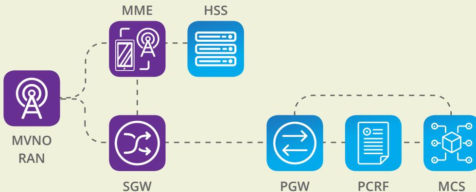
**FIGURE 4. TOPOLOGY OF NETWORK ELEMENT SHARING**
